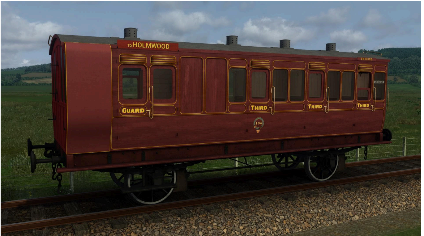
4-wheeled brake third no. 104 in later 1870s condition, still with wooden brake blocks and oil lamps.
